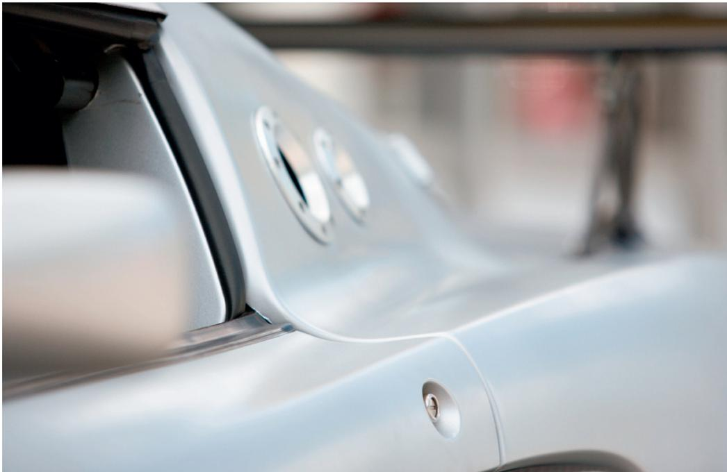
ROHACELL® sandwich elements and fiber materials lower the weight of a car body by 60 to 70 percent compared to the steel parts used until recently.
